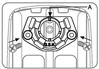
1. Place "A" component on the back cover of the detector and fasten it with two screws.
