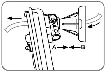
3. Make a hole in the detector's back cover for the installation wire. Run the wire through "A" component inside the detector. Attach the back cover ("A" component ) to "B" component .
