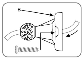
2. Run the installation wire through "B" component. Fasten "B" component to the wall with two screws.
