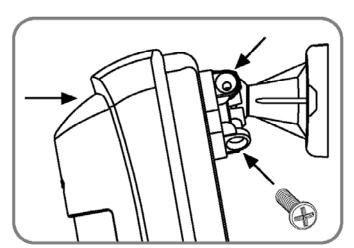
4. Connect the wires to the terminal block and close the detector's cover. Adjust the desirable angle and fix with two screws.
